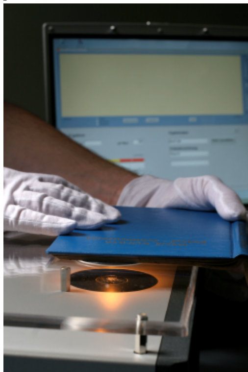
Fig. 1; The SurveNIR instrument for non-destructive evaluation of paper chemical and mechanical properties and for collection surveying, based on chemometric evaluation of NIR spectra.
