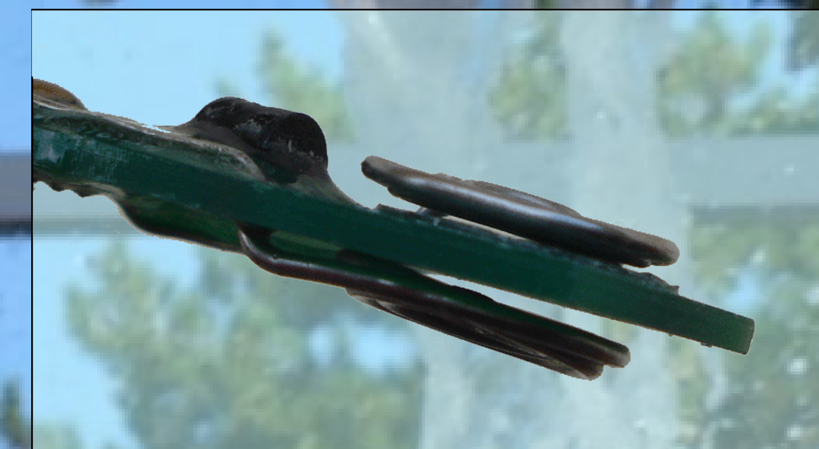
Fig.4, The macro photo of the 2 inox spirals fixed on the two sides of the PCB, the black component is the temperature sensor. To isolate from water all the PCB, excluding the spirals, was immersed 2 times in Araldite resin.
