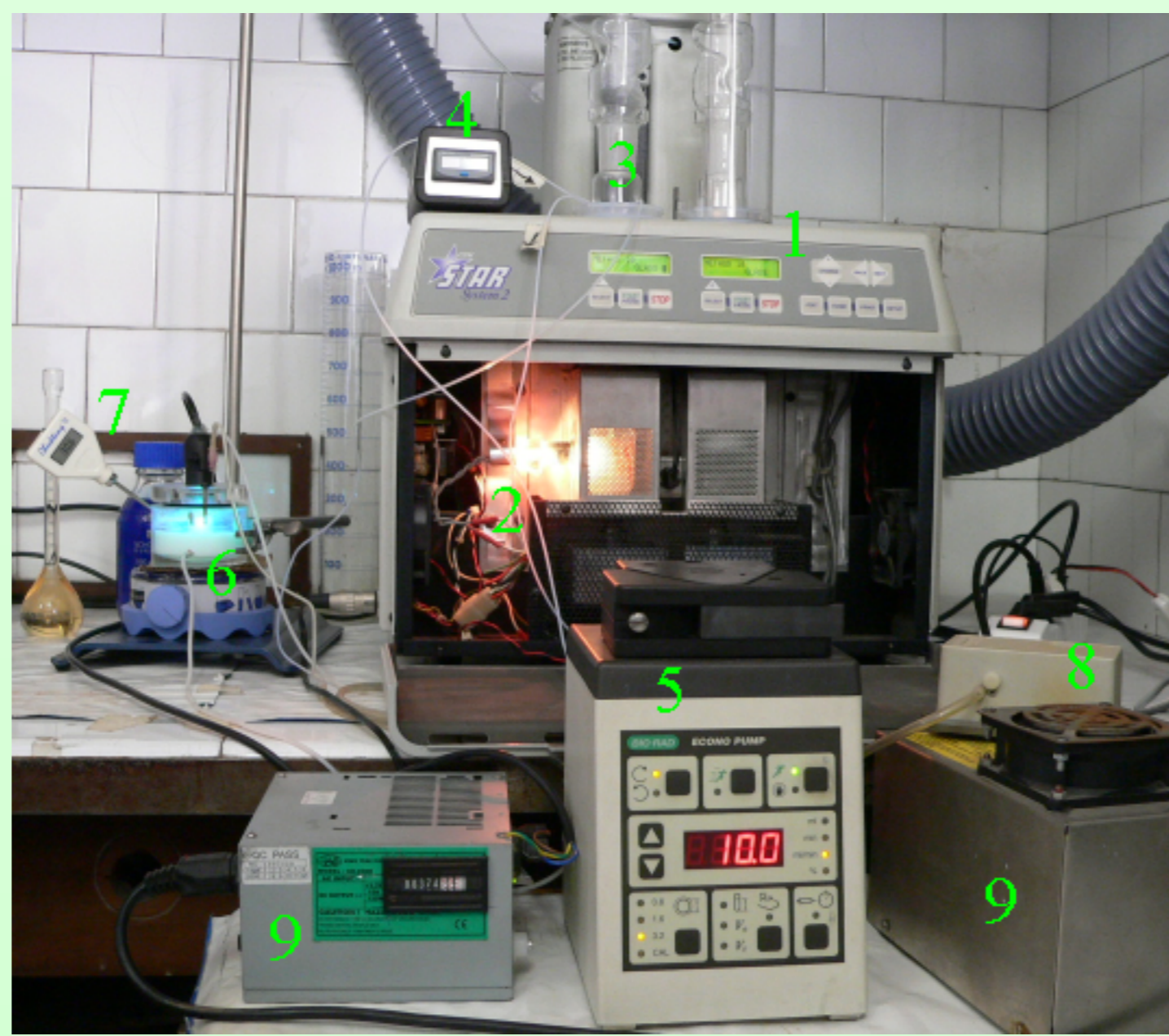
Fig. 7. Photodegradation system: 1= laboratory microwave digesting system modified, by CEM Italy, both in the firmware and hardware to obtain a pulsed operation and also a window needed by the internal lamp; 2= quartz dichroic internal lamp overvoltage in C.C. to obtaining a continuous emission (but with loss of life time) and also "1 sun" (with spectrum, intensity and focusing near the summer sun in the Mediterranean places); 3= fused silica cell with UV-Vis transmittance, volume of 50 mL and holes for the circulation tubing and air flows; 4= counter of magnetron impulses, useful to obtain the reproducibility of the MW supply; 5= dual circuit peristaltic circulation pump, by means of four Teflon tubes it allows circulation of solution (105 mL) in about 6 minutes and maintains the catalyst suspension; 6= the cell in PMMA, above the magnetic stirrer, containing Hg vapors lamp mainly emitting at 254 nm, the thermometer, the stirring bar, a syringe needle for the continuous air insufflation and a hole for sampling during the degradation; 7= the digital thermometer allows to avoid the thermal microwave effect, monitoring the temperature (always under 40^\circ\text{C} ) at different duty cycles; 8= membrane air pump, with splitter, to insufflate the filtered ( 0.47 \mu\text{m} ) room air, by Teflon tubes, in the outside and inside cells, with the triple purpose to remove produced \text{CO}_2 to guarantee an oxygen excess in solution, to keep the catalyst in suspension; 9= two power supplier to feed UV lamp in A.C. and quartz lamp in C.C..
