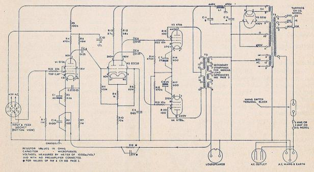
Circuit diagram of Leak TL12 Main Amplifier.
