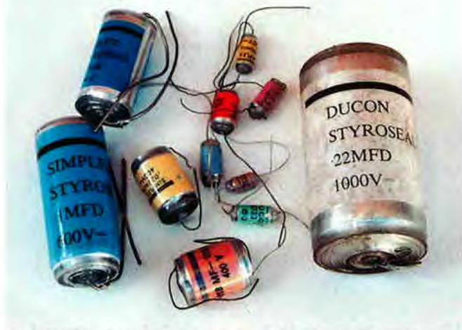
Styroseal capacitors became available around the same time as polyester capacitors and are quite reliable.
