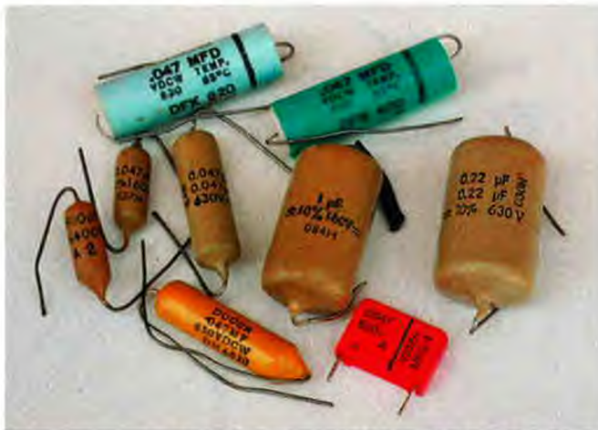
Polyester capacitors became available in the late 1960s, towards the end of the valve era, and are very reliable.
