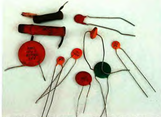
Early ceramic capacitors were not very reliable but later types gave few problems.
