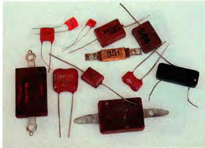
Mica capacitors usually have relatively low values and are typically used as RF bypasses, in tuned circuits.
