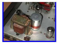
Using the smallest bit possible, drill a hole for each new lead wire next to each terminal it will attach to. Push the leads through the phenolic disk, seating the new electrolytics on the disk. Wrap the leads around their terminals, and route the ground to the can, adding a bit of spaghetti tubing if needed. Solder the new leadouts to the terminals.
