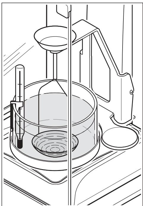
Prepare the balance for the density determination (install draft shield element, bracket, equalizing washer and platform) as described in Section 2.
