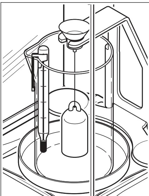
Suspend the sinker (10) from the bracket and ensure that it does not touch either the beaker or the thermometer.
