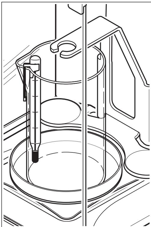
Prepare the balance for the density determination (install the support plate, bracket, and pan) as described in Section 2.
