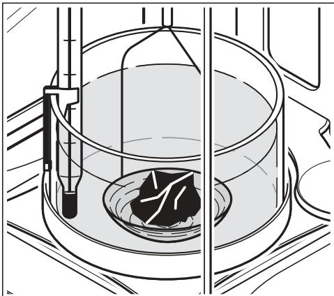
Remove the solid from the pan, close the draft shield doors and tare the balance. Place the solid after in the holder (6). Ensure that no air bubbles adhere to the solid (remove any air bubbles with a fine brush).
